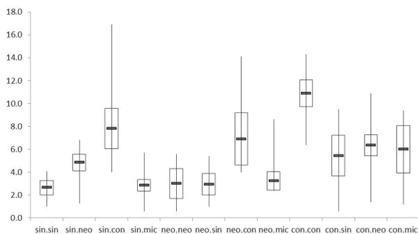
Figure 2. Modified notch box graph with the median (dash), general range (vertical line) and confidence limit (box), for the largest discrepancy values ( $\mu\text{m}$ ) distributed by implant brand and the prosthetic rotational component placed. SIN: SIN Implant Systems, São Paulo; CON: Conexão Sistemas de Próteses, Arujá; NEO: Neodent, Curitiba.
