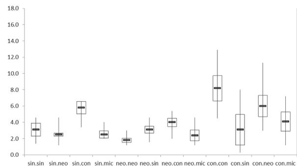
Figure 3. Modified notch box graph with the median (dash), general range (vertical line) and confidence limit (box), for the largest discrepancy values ( $\mu\text{m}$ ) distributed by implant brand and the prosthetic non-rotational component placed. SIN: SIN Implant Systems, São Paulo; CON: Conexão Sistemas de Próteses, Arujá; NEO: Neodent, Curitiba.
